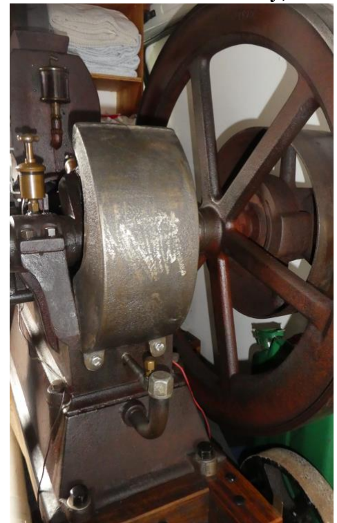
By modifying the pattern, I made for the Jacobson engines I was able to cast a replacement crank guard very similar to the original.
