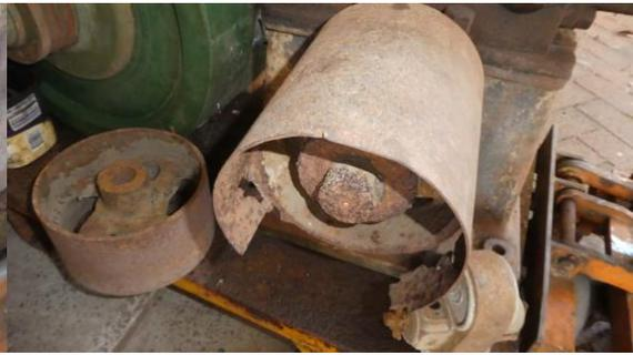
*It had a cast iron pulley with a wide steel strap riveted on for running a fast and loose belt.*
