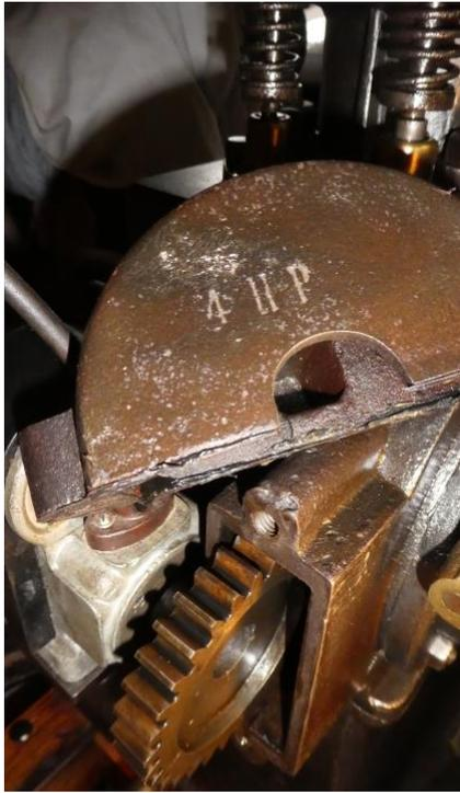
*The magneto drive gear cover marked 4 HP.*
