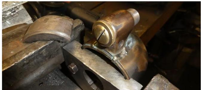
*Carburetor repair jig with the practice body for both straightening and silver soldering.*
